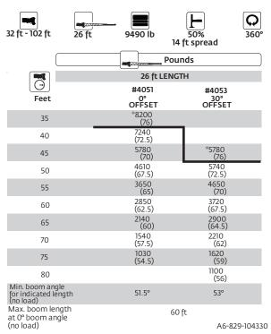
NOTE: () Boom angles are in degrees. #LMI operating code. Refer to LMI manual for instructions. "This capacity based on maximum boom angle.
